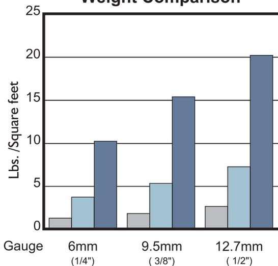
QuickSilver® Durapro® Aluminium Carbon Steel HMW-PE HD-PE
